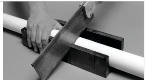
Plastic tubing cutters may also be used for cutting plastic pipe; however, some produce a raised bead at the end of the pipe. This bead must be removed with a file or reamer, as it will wipe the cement away when pipe is inserted into the fitting.
